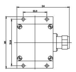
Inset terminations are used in quantitatively absorbing energy of RF and microwave system, they are commonly used as dummy loads of antenna and transmitter.
