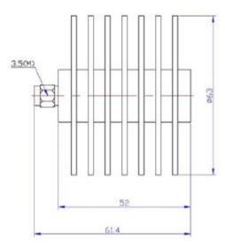
Coaxial fixed terminations absorb RF& microwave energy and are commonly used as dummy loads of antenna and transmitter. They are also used as match ports in many multiport microwave device such as circulator and directional coupler to make these ports which are not involved in the measurement be terminated in their characteristic impedance in order to ensure an accurate measurement.
