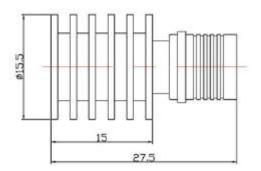
UCL-QT coaxial fixed terminations absorb RF& microwave power and Suitable applications include radio base stations and other radio equipment, especially where high density connector population is required.
