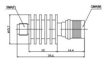
UCL-QSP coaxial fixed attenuators absorb RF& microwave power and suitable applications include radio base stations and other radio equipment, especially where high density connector population is required.
