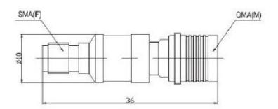
UCL-QSP coaxial fixed attenuators absorb RF& microwave power and suitable applications include radio base stations and other radio equipment, especially where high density connector population is required.
