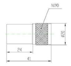
Push-on Coaxial Terminations are mainly used quickly and precise measurement for coaxial system with feature of convenient directly push on or out of test cable.
