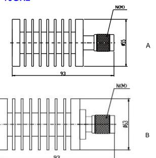
Coaxial fixed terminations absorb RF& microwave energy and are commonly used as dummy loads of antenna and transmitter. They are also used as match ports in many multiport microwave device such as circulator and directional coupler to make these ports which are not involved in the measurement be terminated in their characteristic impedance in order to ensure an accurate measurement.
