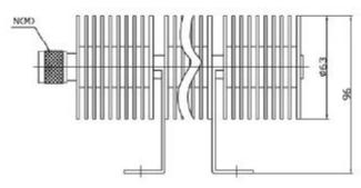
Coaxial fixed terminations absorb RF& microwave energy and are commonly used as dummy loads of antenna and transmitter. They are also used as match ports in many multiport microwave device such as circulator and directional coupler to make these ports which are not involved in the measurement be terminated in their characteristic impedance in order to ensure an accurate measurement.
