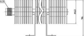
Coaxial fixed terminations absorb RF& microwave energy and are commonly used as dummy loads of antenna and transmitter. They are also used as match ports in many multiport microwave device such as circulator and directional coupler to make these ports which are not involved in the measurement be terminated in their characteristic impedance in order to ensure an accurate measurement.
