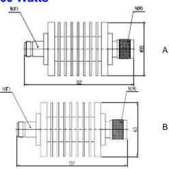
Coaxial fixed attenuators are used in absorbing energy of transmission line, expanding power range and controlling power level, they are also used in accurately measuring power or spectrum of RF microwave transmitters accompany with small power meter, comprehensive tester or spectrum analyzer.
