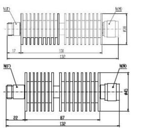
Coaxial fixed attenuators are used in absorbing energy of transmission line, expanding power range and controlling power level, they are also used in accurately measuring power or spectrum of RF microwave transmitters accompany with small power meter, comprehensive tester or spectrum analyzer.
