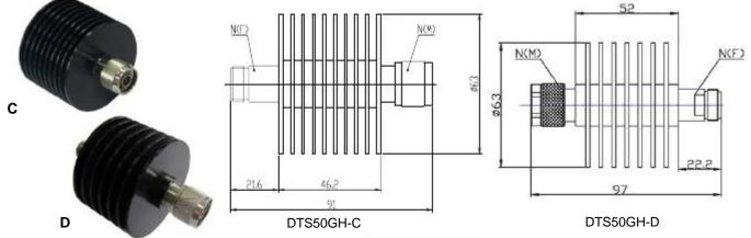
Coaxial fixed attenuators are used in absorbing energy of transmission line, expanding power range and controlling power level, they are also used in accurately measuring power or spectrum of RF microwave transmitters accompany with small power meter, comprehensive tester or spectrum analyzer.
