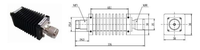
Coaxial fixed attenuators are used in absorbing energy of transmission line, expanding power range and controlling power level, they are also used in accurately measuring power or spectrum of RF microwave transmitters accompany with small power meter, comprehensive tester or spectrum analyzer.
