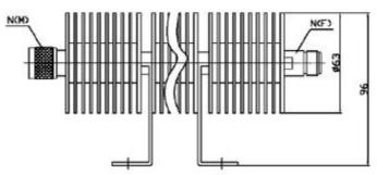
Coaxial fixed attenuators are used in absorbing energy of transmission line, expanding power range and controlling power level, they are also used in accurately measuring power or spectrum of RF microwave transmitters accompany with small power meter, comprehensive tester or spectrum analyzer.
