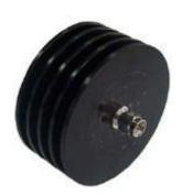
Coaxial fixed attenuators are used in absorbing energy of transmission line, expanding power range and controlling power level, they are also used in accurately measuring power or spectrum of RF microwave transmitters accompany with small power meter, comprehensive tester or spectrum analyzer.
