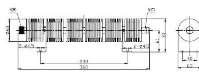
Coaxial fixed attenuators are used in absorbing energy of transmission line, expanding power range and controlling power level, they are also used in accurately measuring power or spectrum of RF microwave transmitters accompany with small power meter, comprehensive tester or spectrum analyzer.
