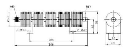
Coaxial fixed attenuators are used in absorbing energy of transmission line, expanding power range and controlling power level, they are also used in accurately measuring power or spectrum of RF microwave transmitters accompany with small power meter, comprehensive tester or spectrum analyzer.
