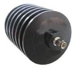
Coaxial fixed terminations absorb RF& microwave energy and are commonly used as dummy loads of antenna and transmitter. They are also used as match ports in many multiport microwave device such as circulator and directional coupler to make these ports which are not involved in the measurement be terminated in their characteristic impedance in order to ensure an accurate measurement.
