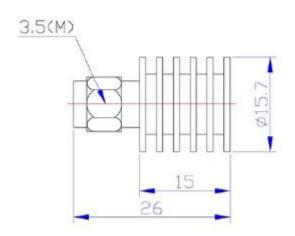
Coaxial fixed terminations absorb RF& microwave energy and are commonly used as dummy loads of antenna and transmitter. They are also used as match ports in many multiport microwave device such as circulator and directional coupler to make these ports which are not involved in the measurement be terminated in their characteristic impedance in order to ensure an accurate measurement.
