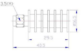
Coaxial fixed terminations absorb RF& microwave energy and are commonly used as dummy loads of antenna and transmitter. They are also used as match ports in many multiport microwave device such as circulator and directional coupler to make these ports which are not involved in the measurement be terminated in their characteristic impedance in order to ensure an accurate measurement.
