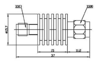
Coaxial fixed attenuators can satisfy almost any requirement where a reduction in power is needed and are used to extend the dynamic range of devices such as power meters and amplifiers, reduce signal levels to detectors and match circuits. Attenuators are also used to balance out transmission lines that otherwise would have unequal signal levels.
