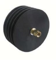
Coaxial fixed attenuators can satisfy almost any requirement where a reduction in power is needed and are used to extend the dynamic range of devices such as power meters and amplifiers, reduce signal levels to detectors and match circuits. Attenuators are also used to balance out transmission lines that otherwise would have unequal signal levels.
