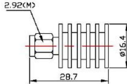
Coaxial fixed terminations absorb RF& microwave energy and are commonly used as dummy loads of antenna and transmitter. They are also used as match ports in many multiport microwave device such as circulator and directional coupler to make these ports which are not involved in the measurement be terminated in their characteristic impedance in order to ensure an accurate measurement.
