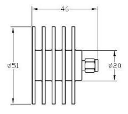
Coaxial fixed terminations absorb RF& microwave energy and are commonly used as dummy loads of antenna and transmitter. They are also used as match ports in many multiport microwave device such as circulator and directional coupler to make these ports which are not involved in the measurement be terminated in their characteristic impedance in order to ensure an accurate measurement.
