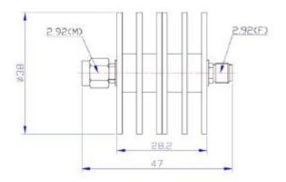
Coaxial fixed attenuators are used in absorbing energy of transmission line, expanding power range and controlling power level, they are also used in accurately measuring power or spectrum of RF microwave transmitters accompany with small power meter, comprehensive tester or spectrum analyzer.
