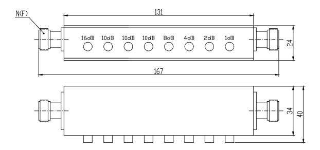
\* Dimensions are given in mm and tolerance  $\pm$  2%.
