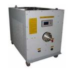
UCL high power water load consists of a 50  $\,^{\Omega}$  RF load assembly, a heat exchange system and a control system, it can be used to absorb max 25-50KW RF energy within DC-800MHz frequency range by releasing RF energy to heat with water cooled method. Further more, the control system can display RF power, water temperature of input and output, and coolant level. It features advanced technology, high power absorbing and facility in use.
