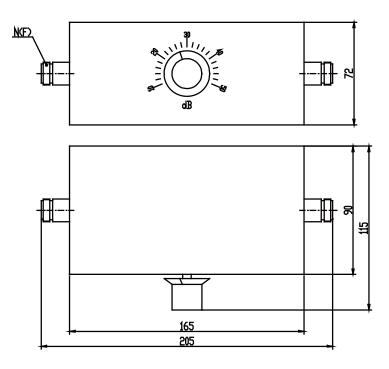
$^{\ast}$  Dimensions are given in mm and tolerance ±2%.
