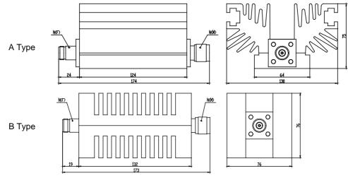
\* Dimensions are given in mm and tolerance  $\pm 2\%$ .
