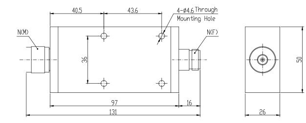
\* Dimensions are given in mm and tolerance  $\pm$  2%.
