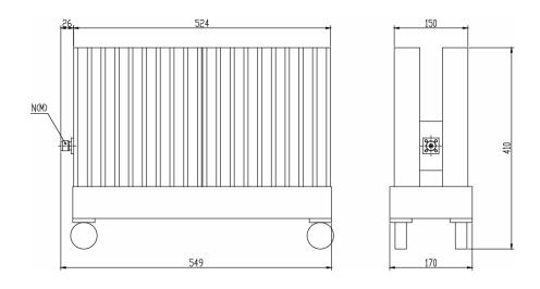
\* Dimensions are given in mm and tolerance  $\pm 2\%$ .
