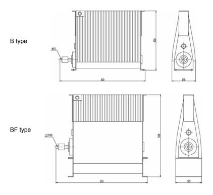
\* Dimensions are given in mm and tolerance  $\pm$  2%.
