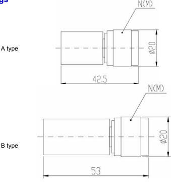
\* Dimensions are given in mm and tolerance  $\pm$  2%.
