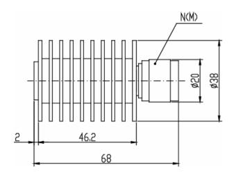
\* Dimensions are given in mm and tolerance  $\pm 2\%$ .
