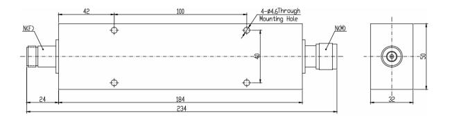
\* Dimensions are given in mm and tolerance  $\pm$  2%.
