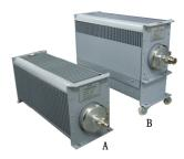
NOMINAL IMPEDANCE:  $50\Omega$ POWER RATING: 2000W continuously PEAK POWER: 50KW AMBIENT TEMPERATURE:  $-40^{\circ}C \sim +45^{\circ}C$ CONNECTOR TYPE: N,L27,7/16 OPERATING POSITION: Horizontal only COOLING METHOD: oil-cooled+ forced draft FINISH: Gray Powder Coat WEIGHT: A: 20kg; B: 23kg PHYSICAL DIMENSIONS: A:  $600 \times 195 \times 260$ mm; B:  $600 \times 195 \times 380$ mm (with fans)
