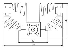
\* Dimensions are given in mm and tolerance  $\pm$  2%.
