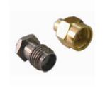
Coaxial fixed terminations absorb RF& microwave energy and are commonly used as dummy loads of antenna and transmitter. They are also used as match ports in many multiport microwave device such as circulator and directional coupler to make these ports which are not involved in the measurement be terminated in their characteristic impedance in order to ensure an accurate measurement.
