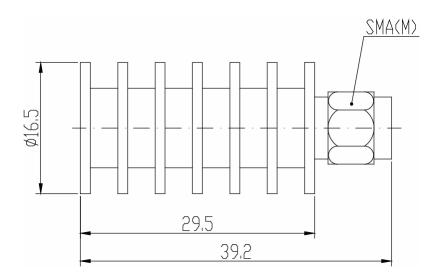
\* Dimensions are given in mm and tolerance  $\pm$  2%.
