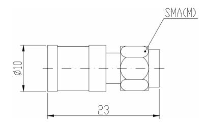
\* Dimensions are given in mm and tolerance  $\pm 2\%$ .
